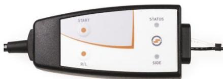
There are two buttons on the RCU: the first (START) has the same function as the START/STOP button on the keyboard; the second button can be pressed to select the side on which the stimulus is presented.
